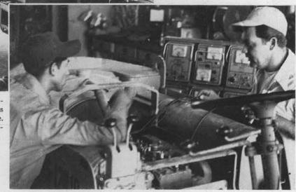
MOTOR ANALYZER leads are run into a fork lift by Charles Garcia as the boss, "Luke" Luker, stops by. If there's anything wrong with the lift's motor or electrical system the analyzer test guages will find it.
